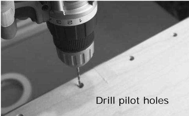
\_\_\_\_E. With the front piece in place - drill 2 pilot holes on opposite sides of the front. Put in 2 of the 1" screws to keep the front from moving while you drill the rest of the pilot holes.
